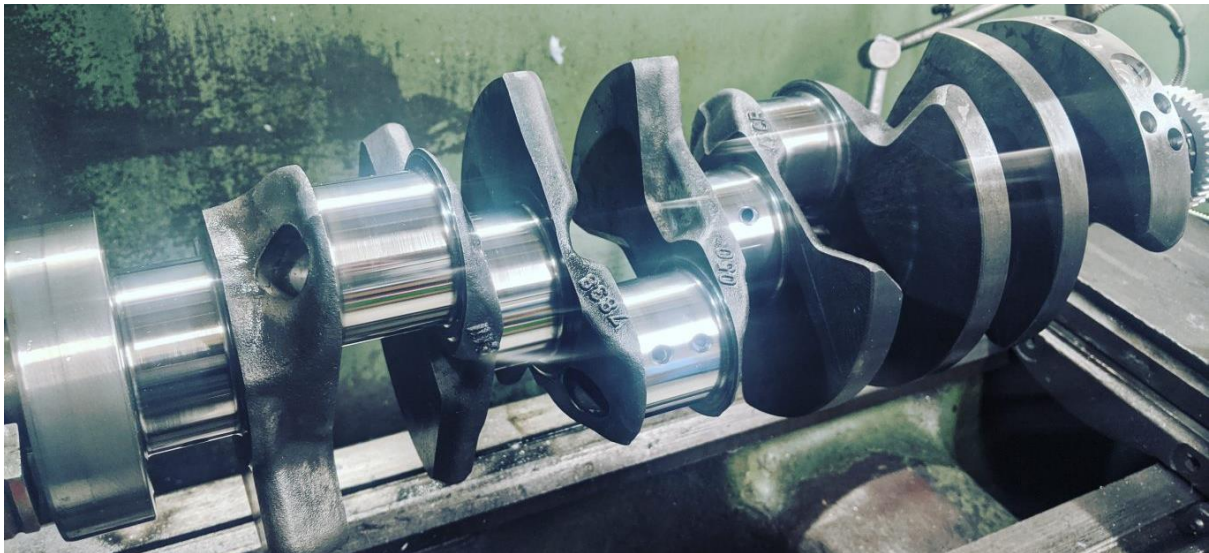
Figure 27 - Forged crank on lathe (Koflach, 2019)
