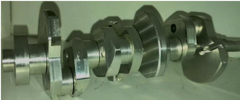
Figure 49 - Aluminium CNC crossplane crankshaft from CAD
