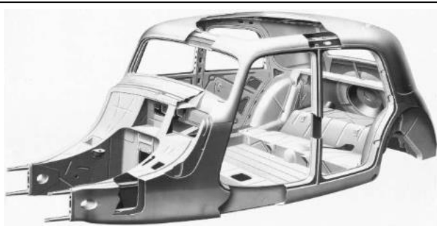
Figure 2.2: World's first Integrated vehicle structure Citroën 11CV: 1934 – 1956
