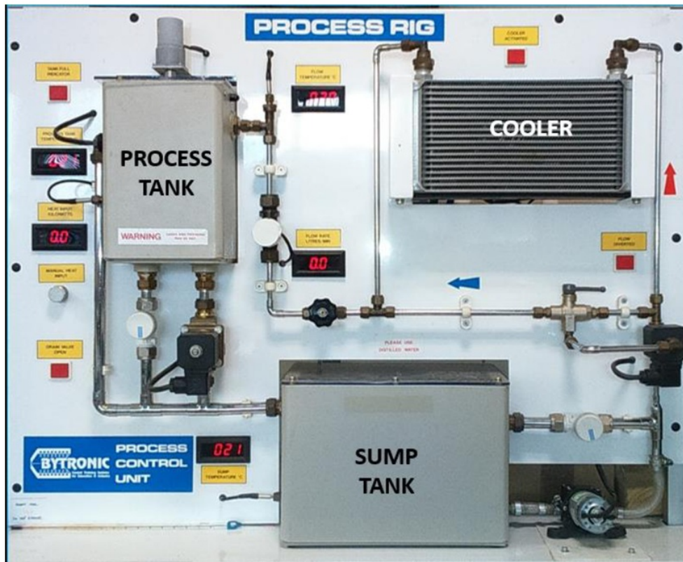
Figure 1: Overview of the Bytronic Process Rig
