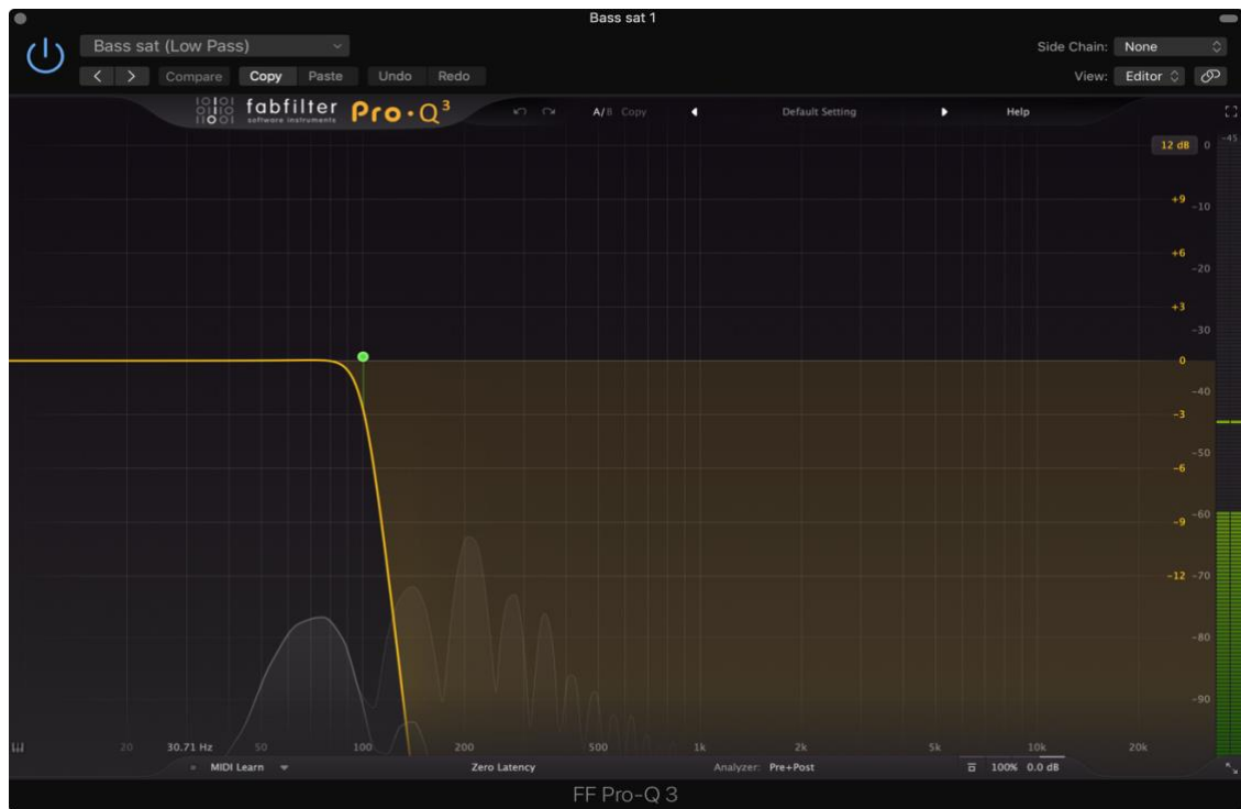
Saturation EQ (B) Low pass filter cutting everything above 100hz
