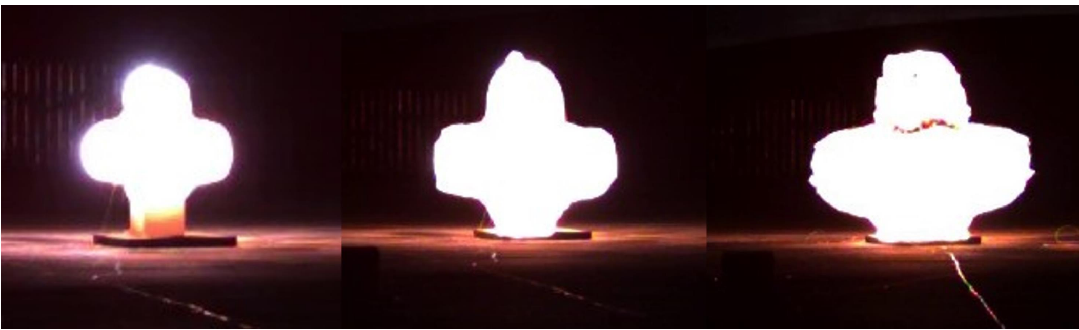
Figure 3: High-speed imaging showed the cruciform fireball development
