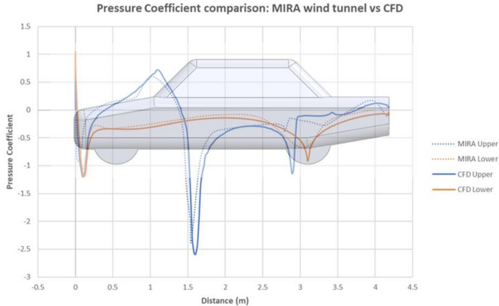
Figure 10. Cl plot comparison: MIRA wind tunnel vs CFD
