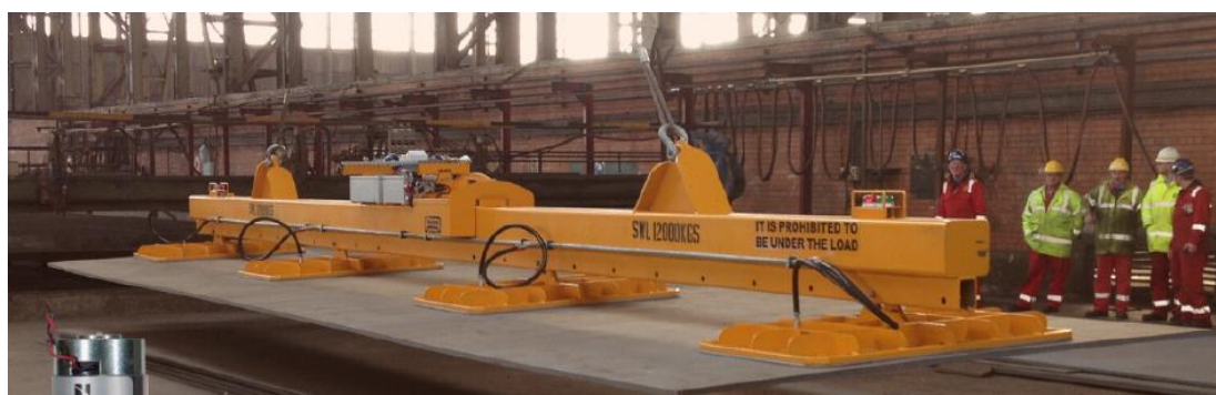
Figure 19: Steel plate vacuum lifting system (Dynaflor, 2022).
