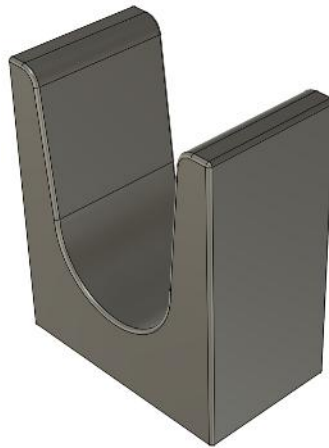
Figure 33: Tapered saddle concept design for end-effector/part alignment.
