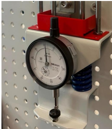
Figure 2. Dial Indicator adjusted to read zero.
