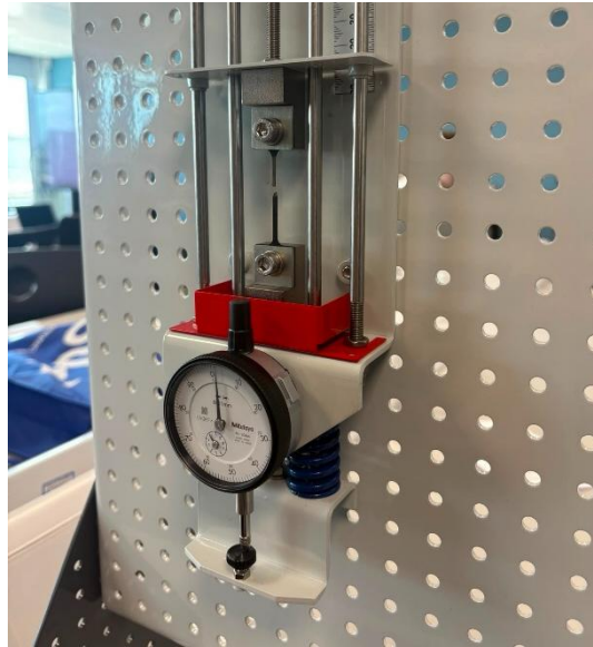
Figure 4. PVC specimen after snapping.
