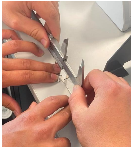
Figure 5. Measuring the final gauge length of aluminium specimen.
