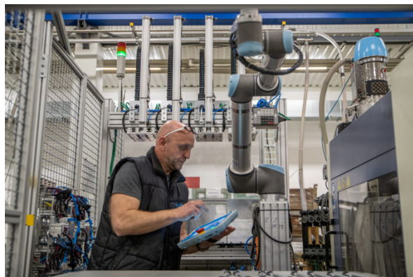
Figure 2 - Cobot assisting a worker with injection moulding [4]
