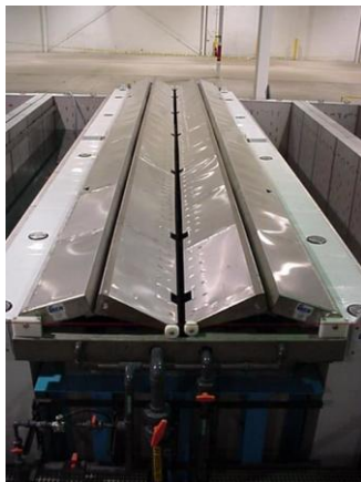
Figure 3 Image showing the folding mechanism of an anodization tank, Products Finishing. 2011.
