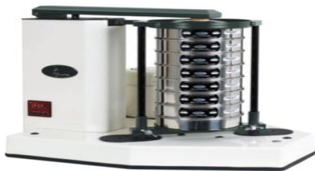
Fig.26. Image of Rotap machine used for measuring particle size in a sample. [50]
