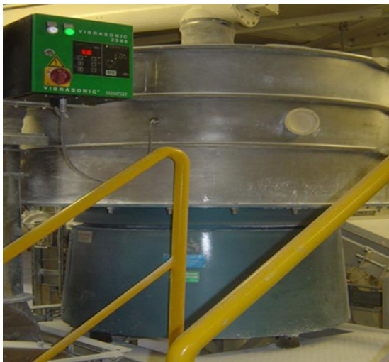
Fig.13. VDS used with separator machine. [30] Fig.14. Spiro screen connected to VDS. [31]
