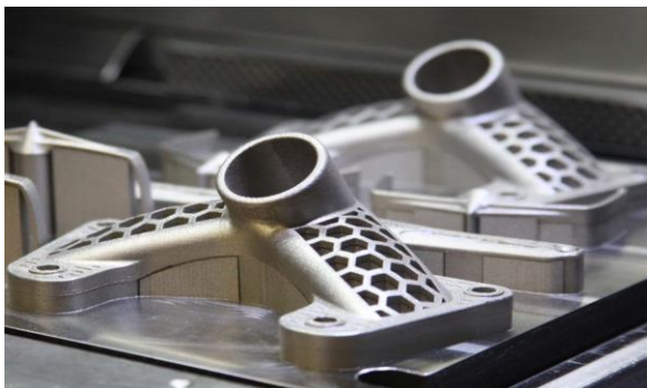
Fig.9. Parts made from direct metals sintering (DMLS). [26]
