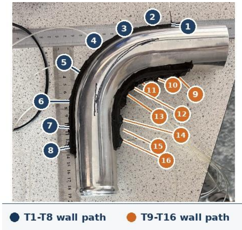
Figure 1. Pressure-tap layout on the 90° bend.
