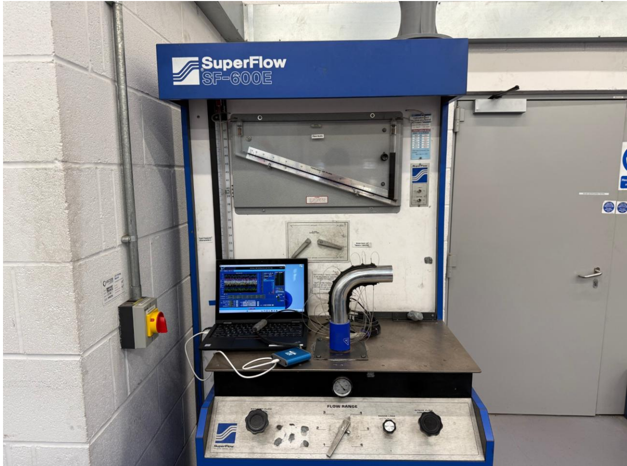
Figure A1. Flow-bench setup for the pressure-tapped 90° pipe test, showing the SuperFlow SF-600E, test piece, pressure-scanner connections and data-acquisition equipment.
