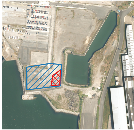
2 - Specifc location of survey area - carried out by adding polygon layers to identify the area (Blue) and also the area unable to survey from the ground body of water (Red).
