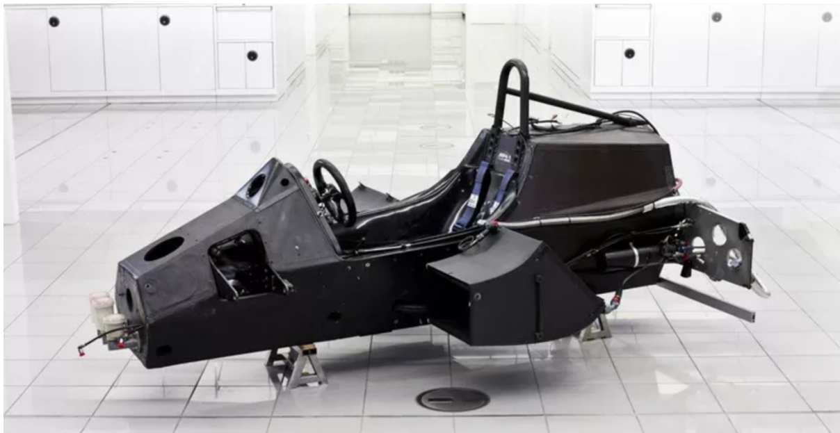
Figure 2 The McLaren MP4 carbon fibre monocoque (Piola)
