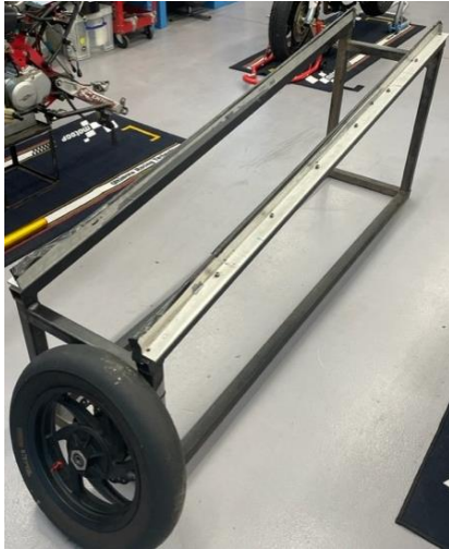
Figure 7 - Experimental setup for measuring front and rear wheel inertia.
