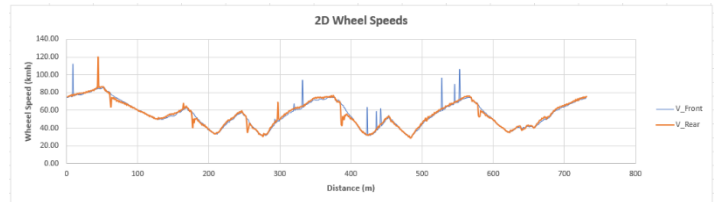
Figure 18 - Front (blue) and rear (orange) wheel speed traces from the exported 2D lap of Kinsham Raceway. Values are measured in Kmh.
