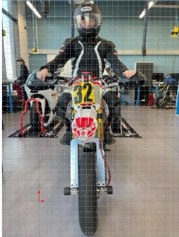
Figure 11 - Frontal area image with transparent grid overlayed for calculations.
