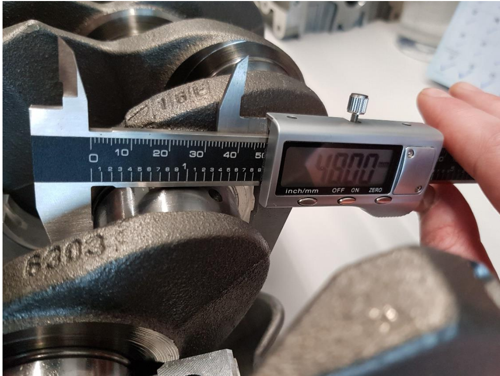
Figure 55 – Measuring The Diameter Of The Crank Journal (Anderson, 2020)
