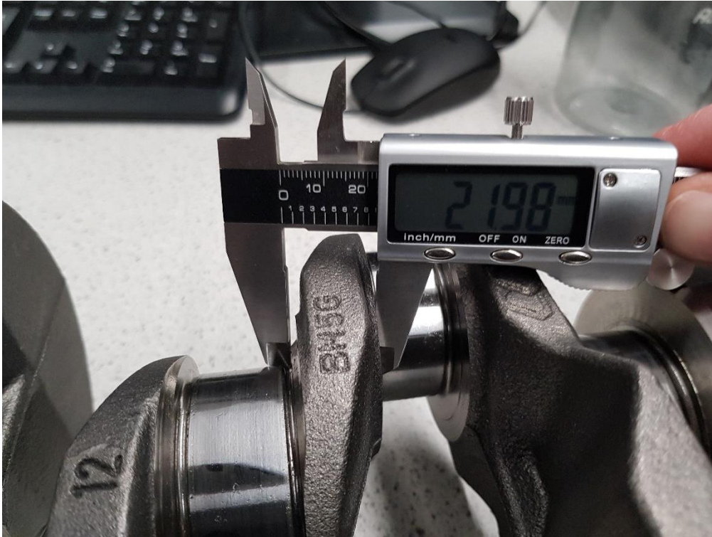
Figure 54 – Measuring The Angled Distance From Point 'A' to 'B' (Anderson, 2020)
