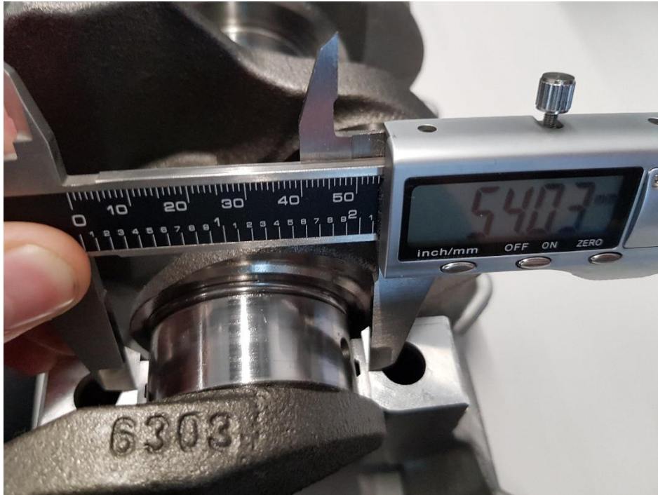
Figure 59 – Measuring The Diameter Of The Crank Journal Bearing Shell (Anderson, 2020)
