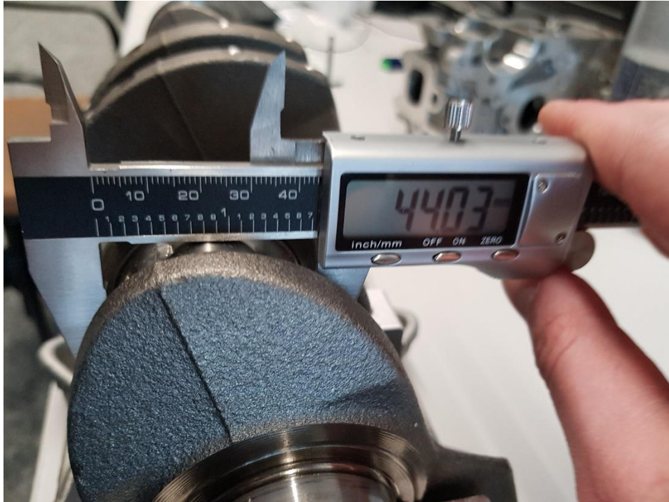
Figure 57 – Measuring The Diameter Of The Big End / Crank Pin (Anderson, 2020)
