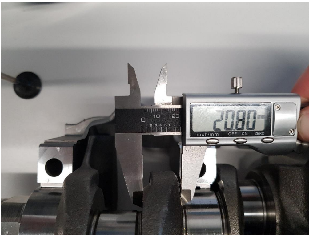
Figure 53 – Measuring The Horizontal Distance From Point 'A' To 'B' (Anderson, 2020)
