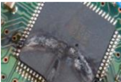
Figure 6: Electrostatic Discharge Damage on PCB (Technofaq, 2018)
