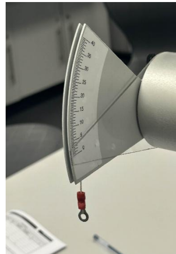
Figure 2 - Rotating chuck with torque arm, and cursor
