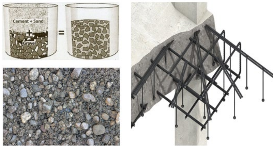
Figure 4: The phenomenon of concrete and the reinforcement of concrete by steel re-bars.
