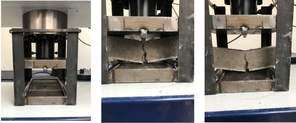
Figure 14: The flexural testing machine employed in the current project.
