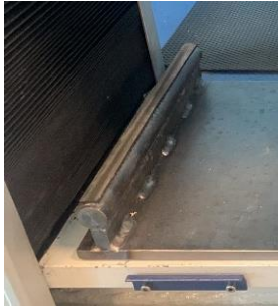
Figure 32 Jig support with rubber applied.
