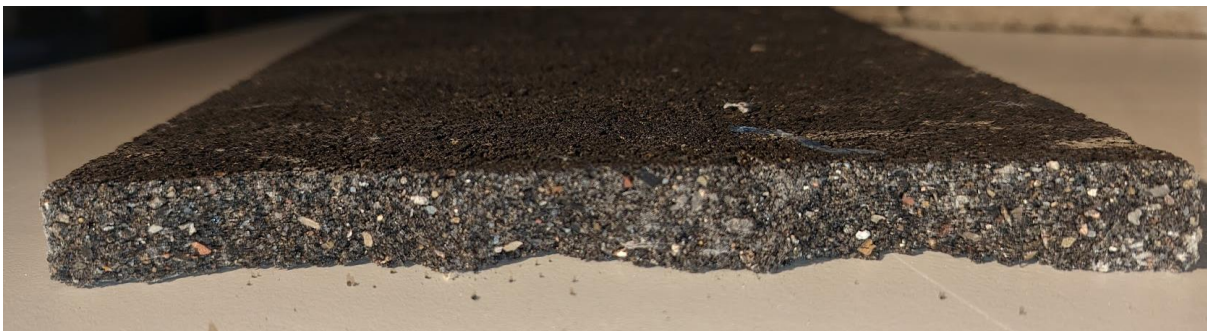
Figure 47 Breaking edge of graphene Art of Eco sample.
