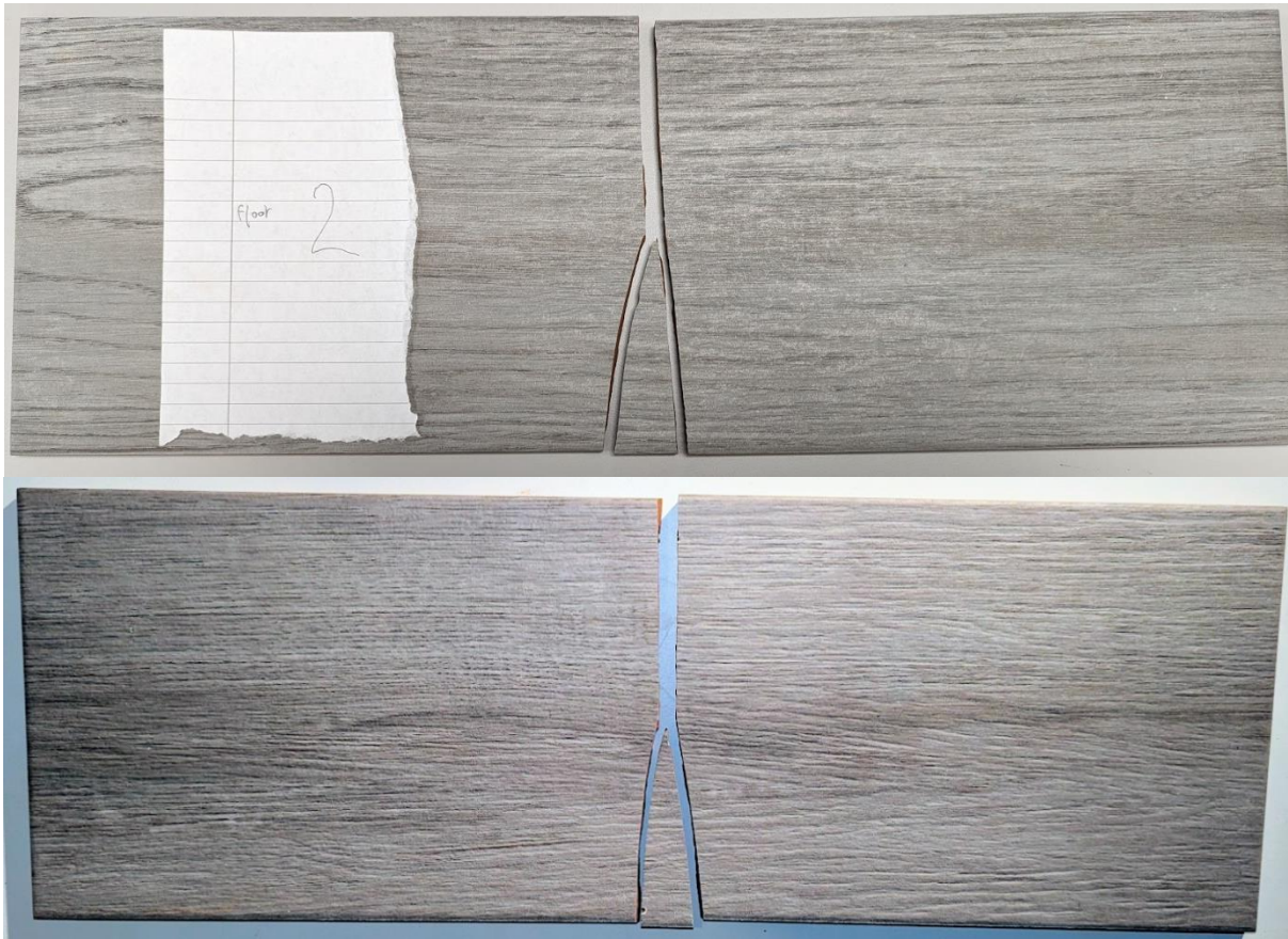
Figure 40 Ceramic floor tiles after failure
