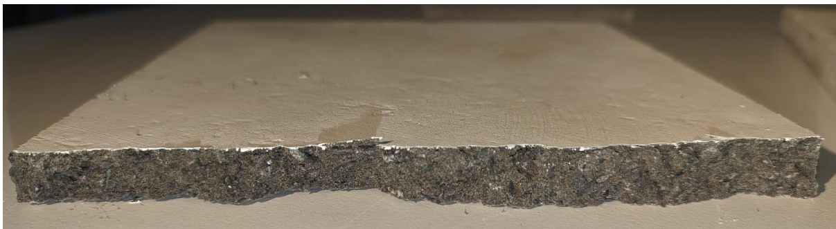
Figure 48 Breaking edge of standard Art of Eco sample.
