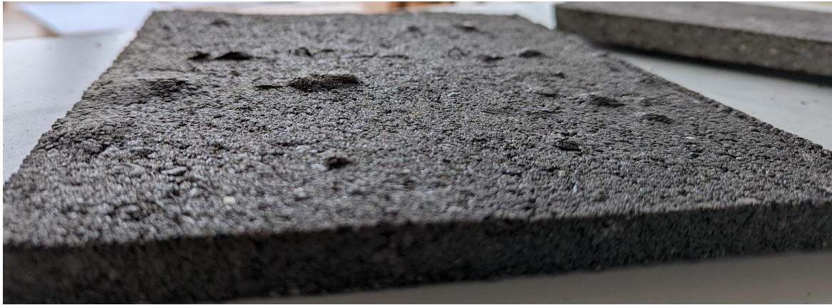
Figure 34 Graphene sample with imperfections
