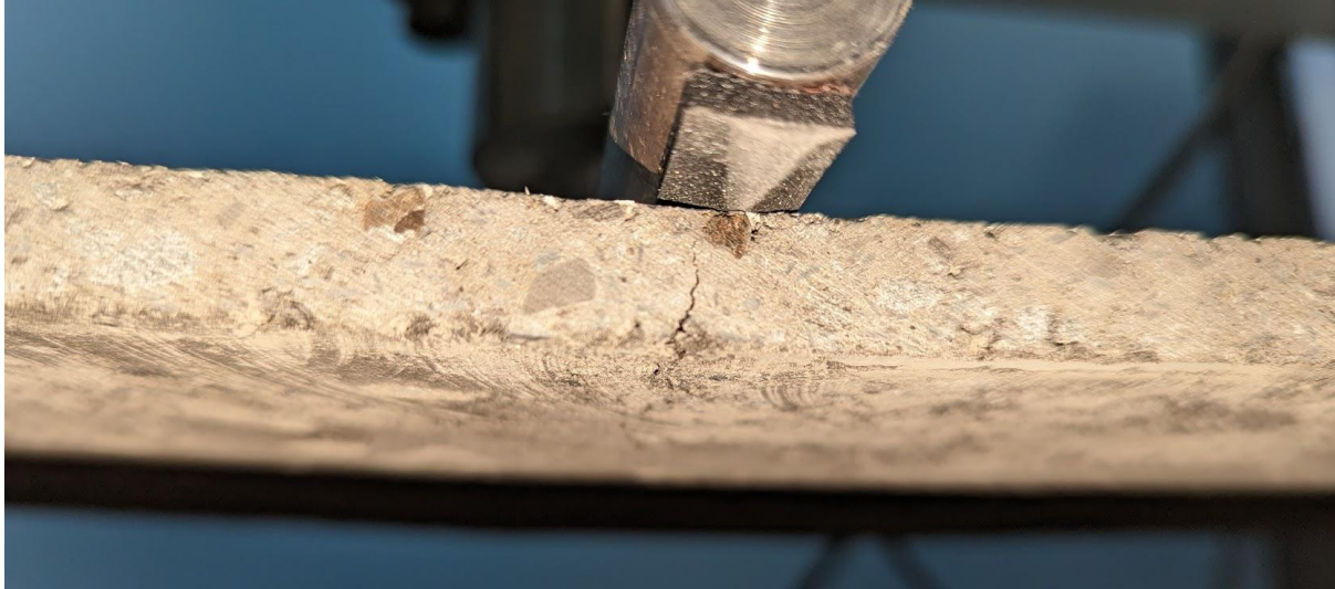
Figure 43 Crack developing in a standard Art of Eco sample.
