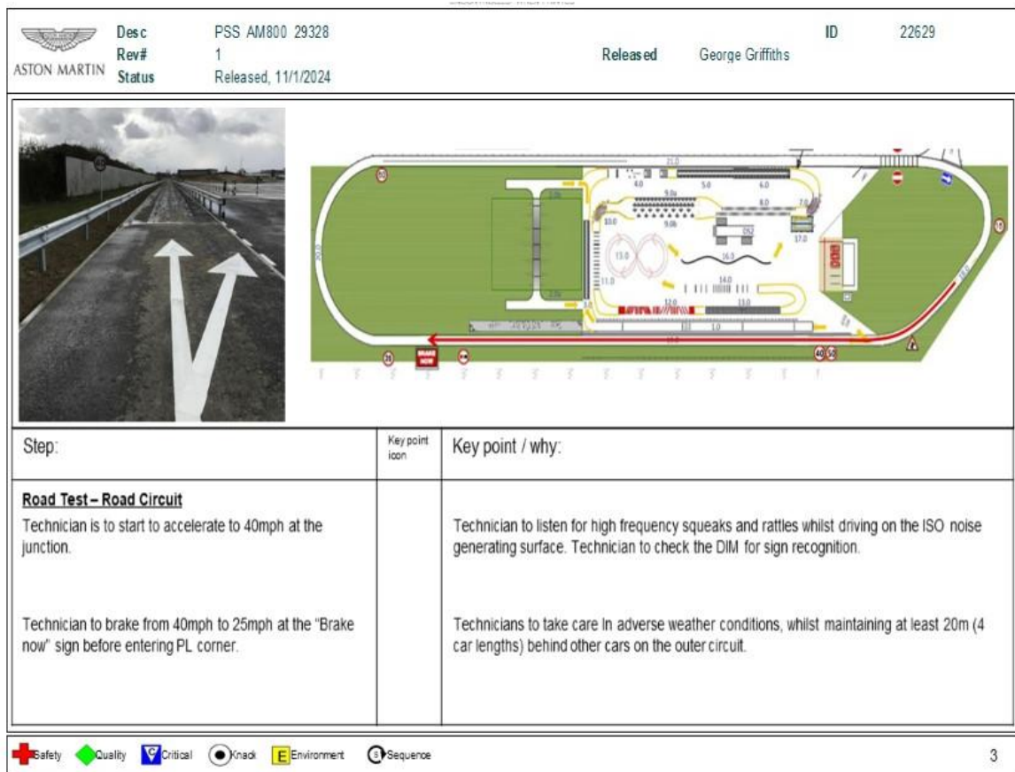
Figure 3- Current process document for the NVH detection process (Aston Martin, 2026)
