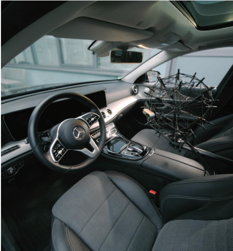
Figure 8-Acoustic camera used in a vehicle for interior testing (GFAI tech, 2026)
