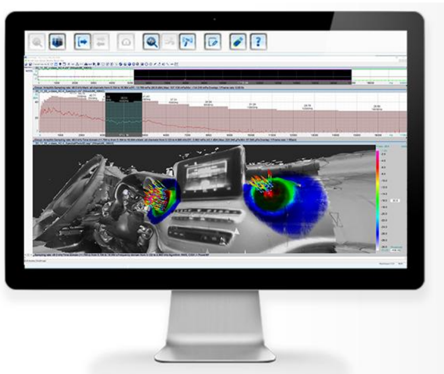
Figure 7-Noise Image Analysis Software for Acoustic Imaging Beamforming 3D (GFAI tech, 2026)
