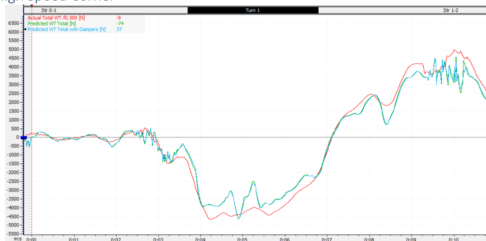
Graph 16 – Weight Transfer comparison equations – high speed corner
