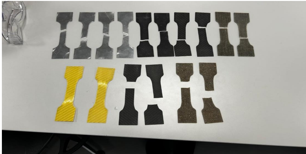
Figure 9 Post Tensile test fractures of each material tested
