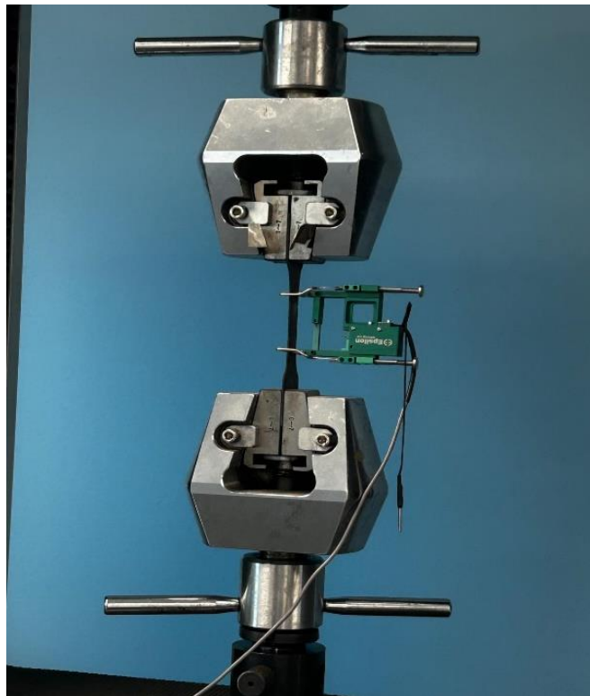
Figure 3 showcasing an example of a specimen in the tensile test machine
