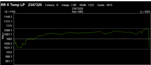
Fig 5 – Example of a temperature trace within range
