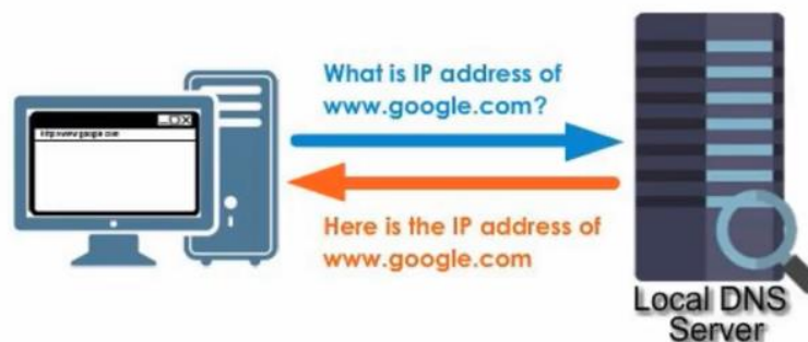
Figure 8: Local DNS server responses to DNS client
