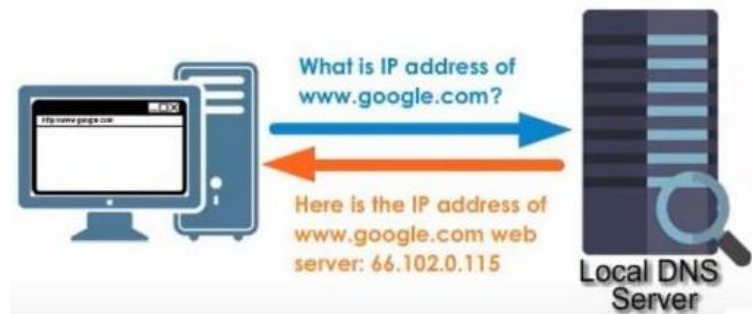
Figure 10: Local DNS server returns response to DNS client
