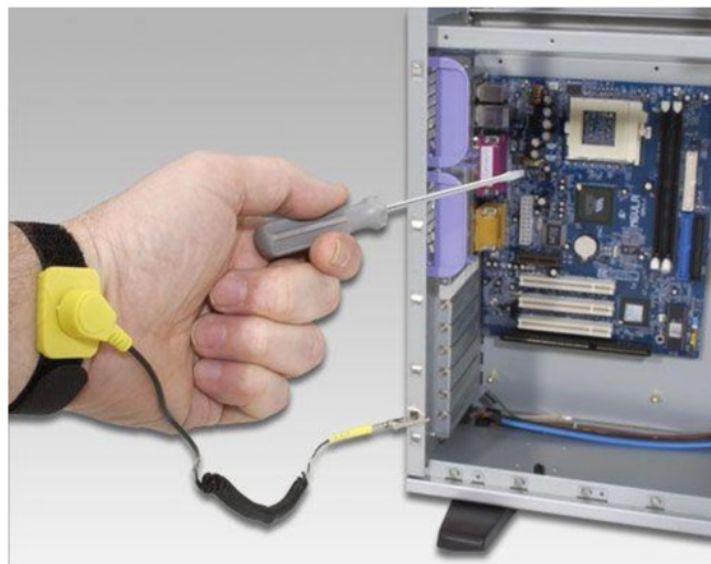
Figure 9 - Technicians Earthing Strap
