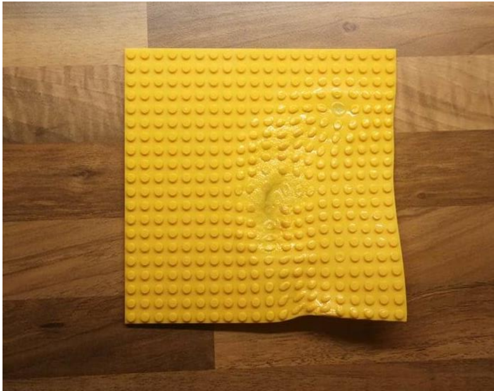
Fig.1.1.4. ABS after being exposed behind the stove for over an hour.
