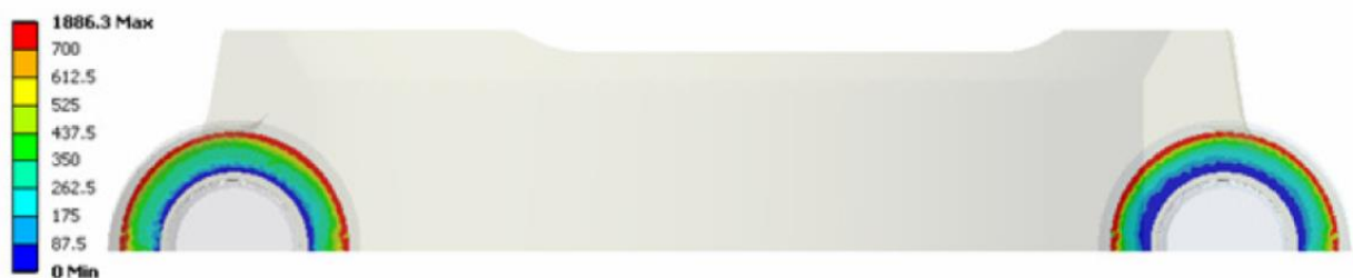
Figure 10 - Connecting Rod Bolt to Cap Clamping Force (De Lima E Silva, 2010)
