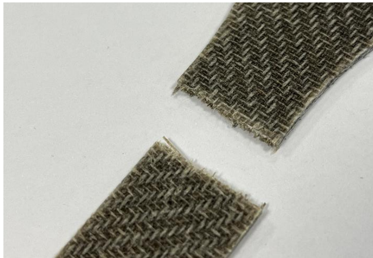
Figure 20 - Flax Woven Sample Failure Point
