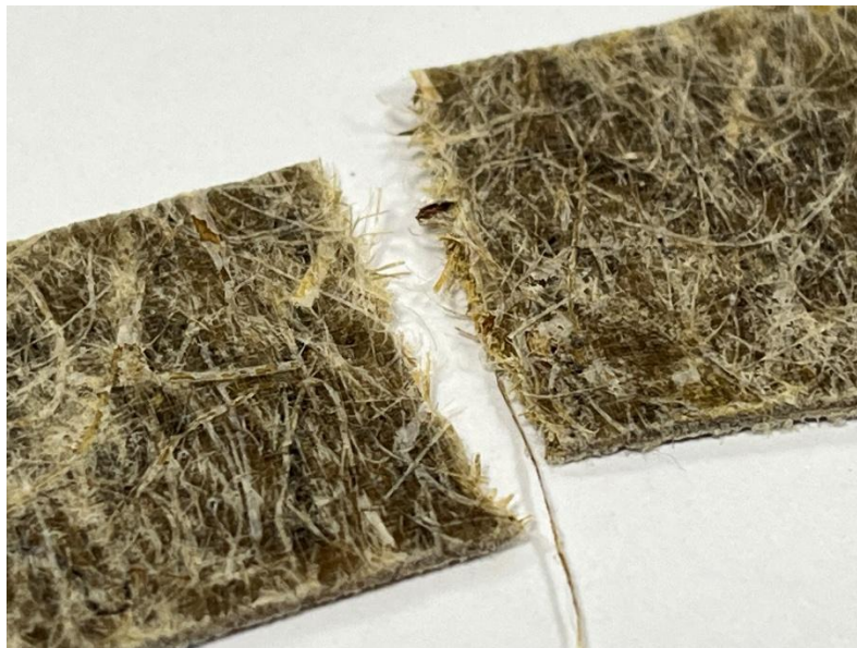
Figure 10 - Hemp (Bio Resin) Sample Failure Point
