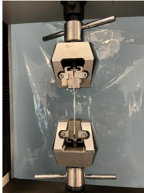
Figure 4 - Gripping Configuration for Tensile Testing
