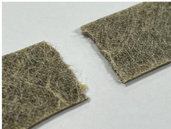
Figure 18 - Flax Non-woven Sample Failure Point
