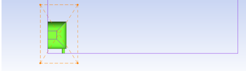
Figure 9. Density box viewed from the front face of the Ahmed body.
