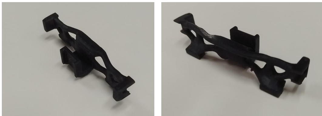
Figure 11 3D Printed Prototype using Generative Design Model
