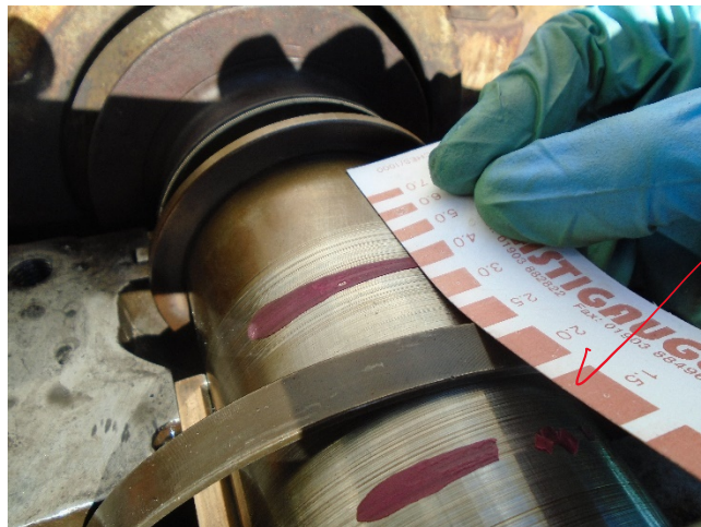
Figure 4 - White Metal Bearing Clearances Being Checked as Part of A Turbine PM
