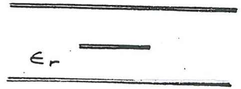
Stripline (Triplate) give better shielding
