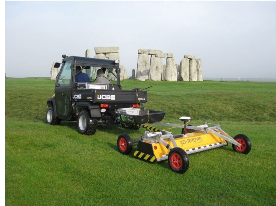
Multi-channel vehicle towed ground penetrating radar (GPR) system in operation at Stonehenge. © Historic England - Geophysics Team
