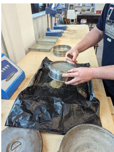
Figure 43 – Removal of sample from sieve pan
