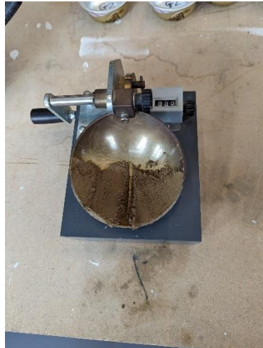
Figure 23 – Soil Sample LL1 in Casagrande Cup Apparatus
