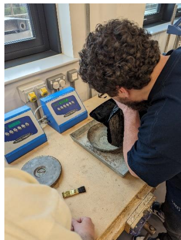
Figure 44 – Pouring of sample post-vibration into metal Pan.
