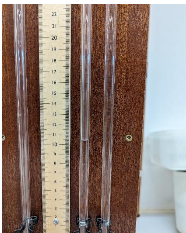
Figure 36 – Sample 2 Manometer Faulty Reading
