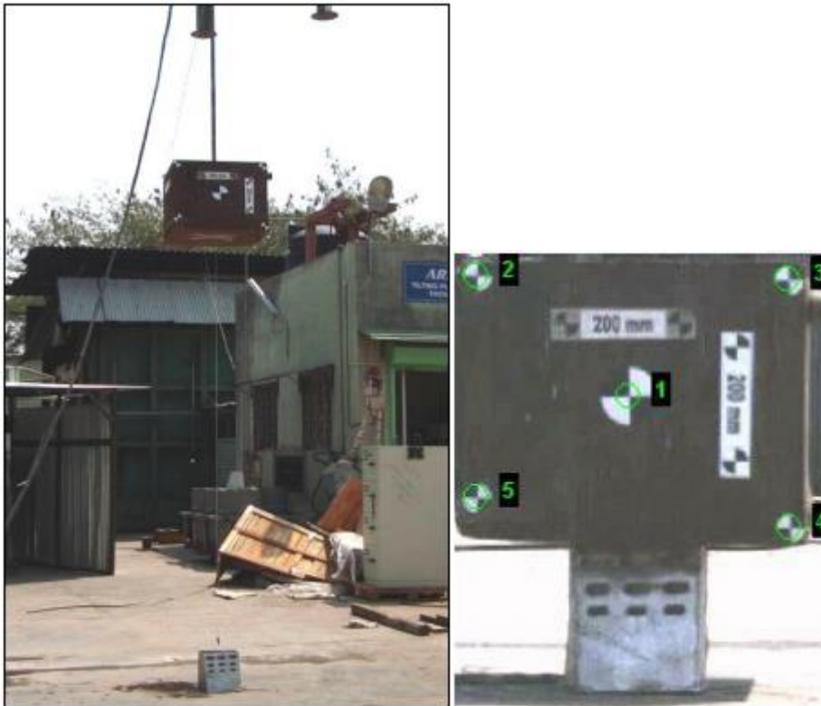
Figure 3: Drop testing crash structure(Kumar et al. , 2012)
