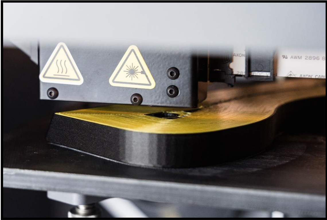
Figure 10. Carbon-Fibre 3D Printing (3D Printing Carbon Fiber and Other Composites, 2022)
