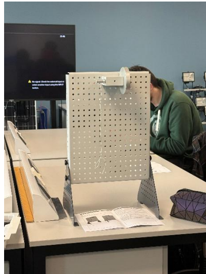
Figure 1 – Flywheel and block bearing attached to work panel
