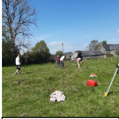
Image 41b: Using the dumpy level to get the height above sea level (Own Image, 09-05-2025).
