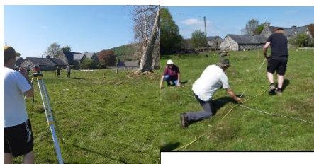
Image 18: Setting up the dumpy level across from the tree (Own Image, 02-05-2025).
