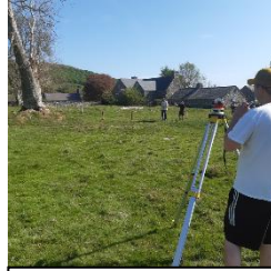
Image 41c: Using the dumpy level (Own Image, 09-05-2025).
