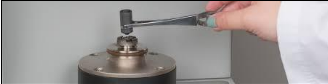
Figure 13 - Loading Graphite Crucible (LECO, 736 Series Inert Gas Fusion analysis of Oxygen and Nitrogen, 2026)
