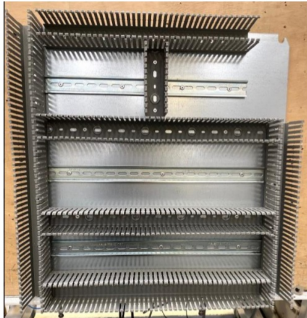
Figure 36 – Panel Trunking Layout
