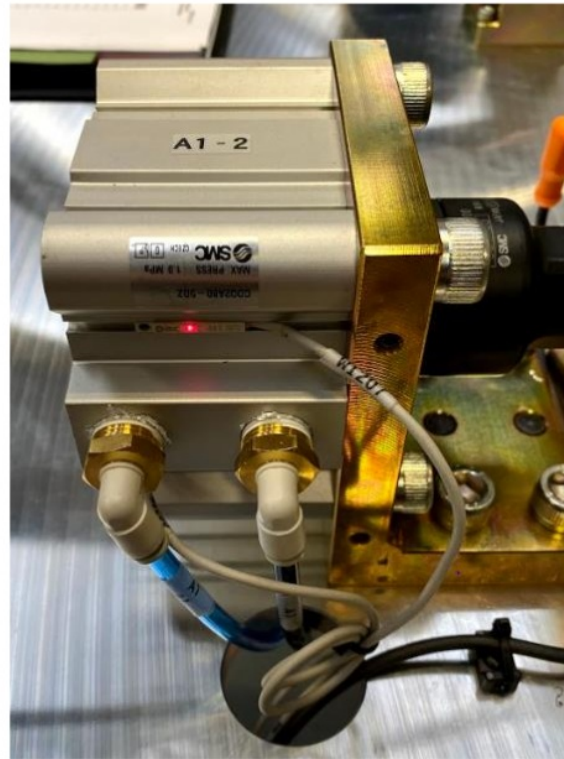
Figure 82 – Dimpling Cylinders with Reed Switches
