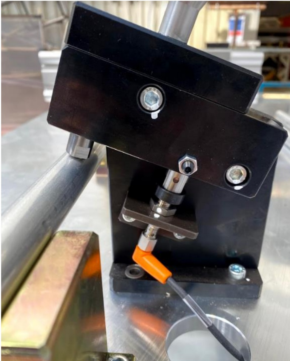
Figure 84 – Hole Aligned sensor on
