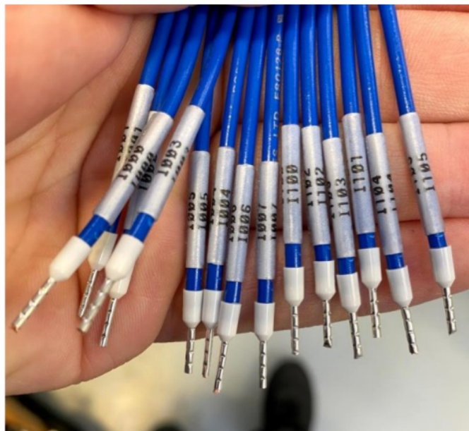
Figure 44 – Input Wires Labelled
