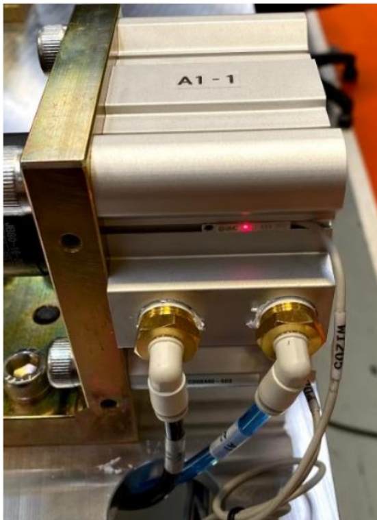
Figure 82 – Dimpling Cylinders with Reed Switches
