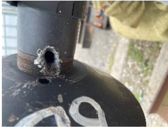
Figure 7 Fragmentation Damage To Pressure Sensor One
