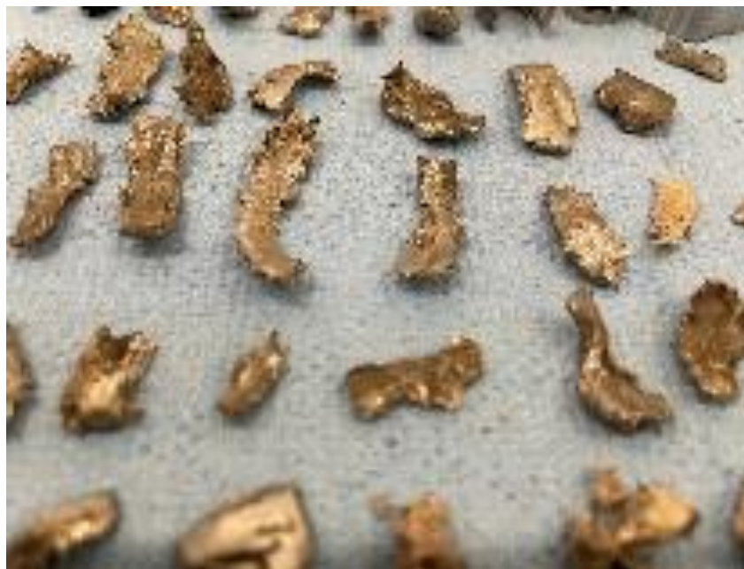
Figure 2 Recovered Post-Blast Fragmentation
