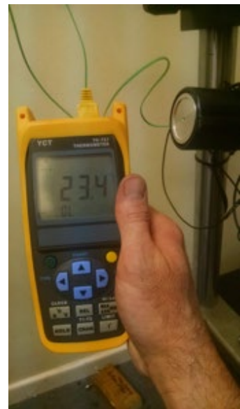
Figure 113, oil temperature reading
