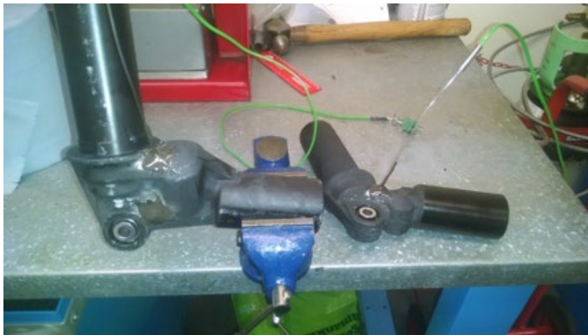
Figure 125, 2013 and 2011 shock absorbers with thermocouples installed
