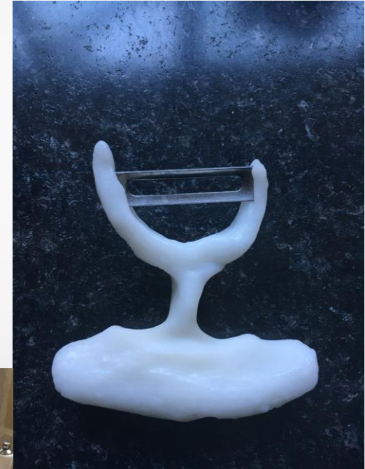
New Peeler Type 2 Prototype material: Multimorph thermoplastic, metal peeler blade Weight: 49g
