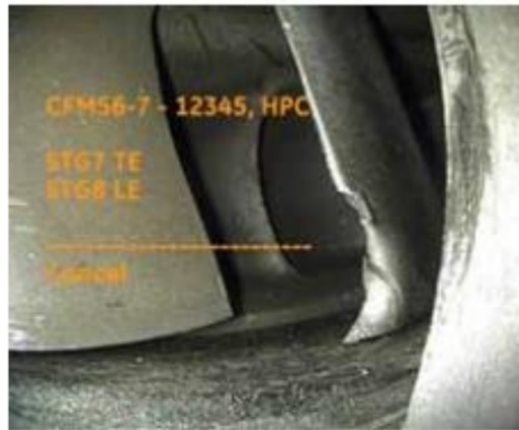
FIG. 3. Defect observed in aircraft engine blade (GE, 2012)
