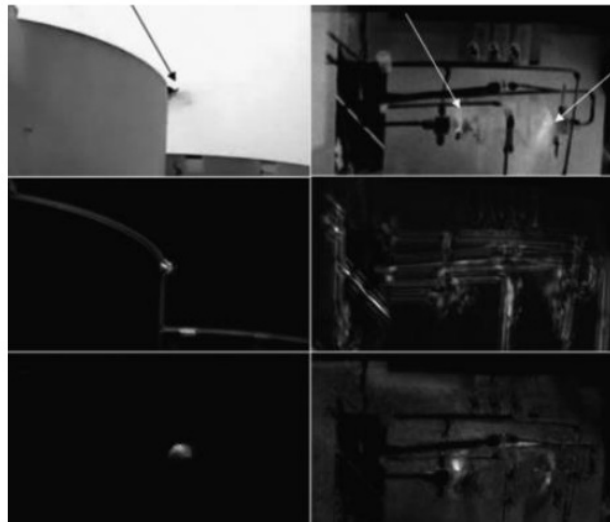
FIG. 15. Infrared camera to detect leaks in tanks and pipes (Zhou & Zeng, 2007).
