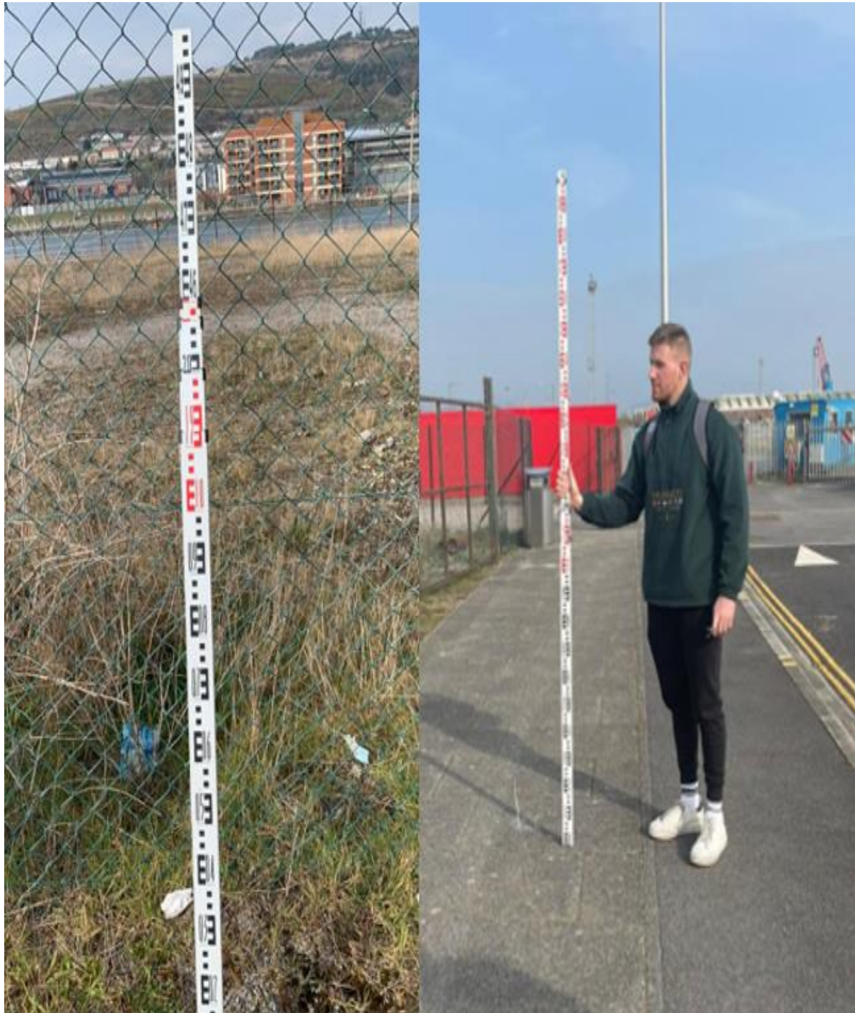
Figure 6: Level staff used on site to take measurements.
