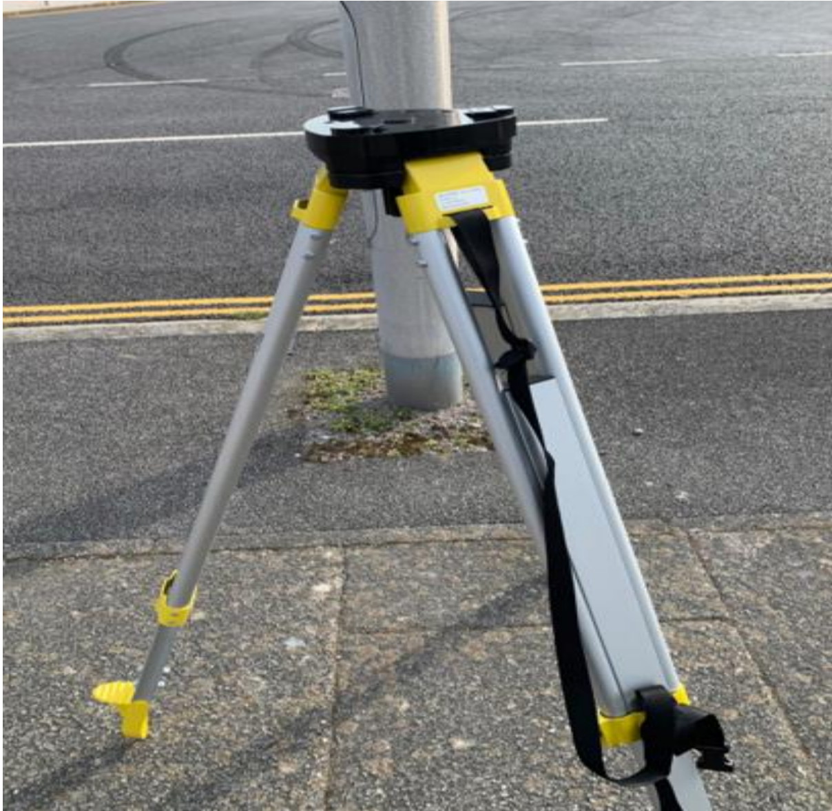
Figure 8: Tripod that was used to install the dumpy level on top of it. The legs of the tripod were extended so the dumpy level would be higher.
