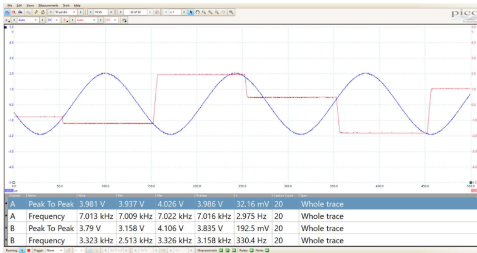
Figure 31 Effect of changing the input frequency in 1kHz at 7KHz
