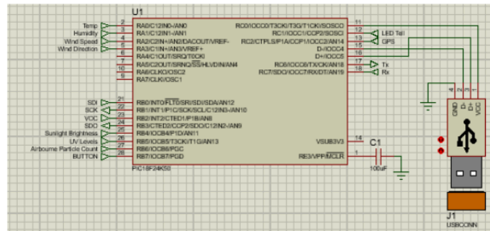
Figure 8 - PIC18F24K50 Proteus Diagram
