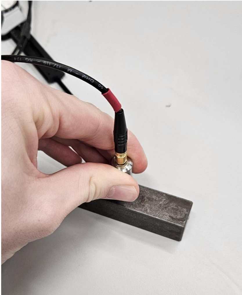
FIGURE 9 MILD STEEL BLOCK WITH 5MHZ PROBE DURING THE EXPERIMENT
