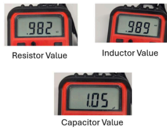
Figure 6: The values of the resistor, inductor and capacitor shown at 982 Ohms, .989 mH and 1.05 \mu f respectively.
